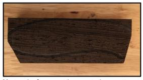
**Note:** before cutting out the pattern, place the tang over the top of the pattern as a reference to ensure the pattern will not cut into the tang opening in the center layer. After your pattern is drawn, insert the blade into the handle to visualize how the knife will look in its finished state.
